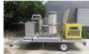
▲ 10 kW Movable Agriculture and Livestock Waste Gasification Power System/10 kW 移動式小型農牧廢棄物氣化發電系統
