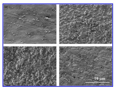
2 Surface image of vinyl siding. *a* Initial; *b* QUV accelerated weathering for 1920 hours; *c* QUV accelerated weathering for 2880 hours; *d* outdoor weathering for 17 years
