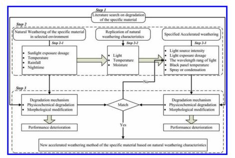
4 New accelerated weathering method of the specific material based on the natural weathering characteristics
