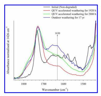
1 Fourier transform infrared spectroscopy-attentuated total reflectance spectra of vinyl siding after accelerated weathering for 0 h (initial), 1920 and 2880 hours and outdoor weathering for 17 years
