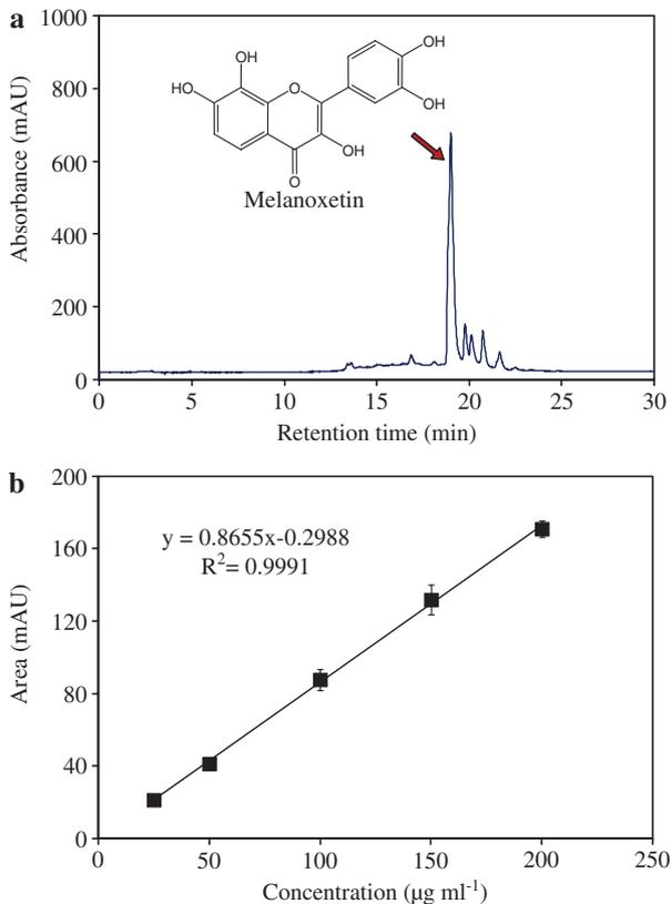
**Figure 3** (a) HPLC chromatography profile of *Acacia confusa* methanolic heartwood extract (detection at 370 nm). (b) The absorption peak area at 370 nm is plotted against the concentration of melanoxetin. Three replicates were made for each test sample.
