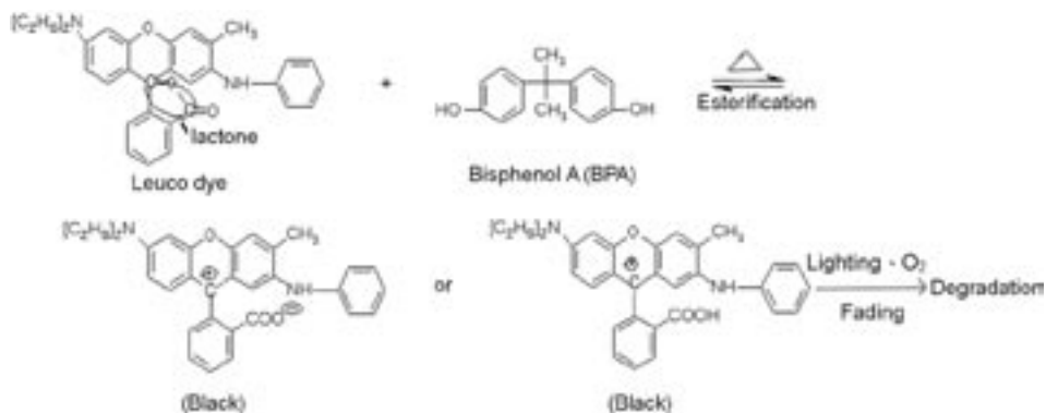
Fig. 2. Reactions of the leuco dye during color rendering. (Hiraishi 1990, Kaneko and Kobayashi 1995).
