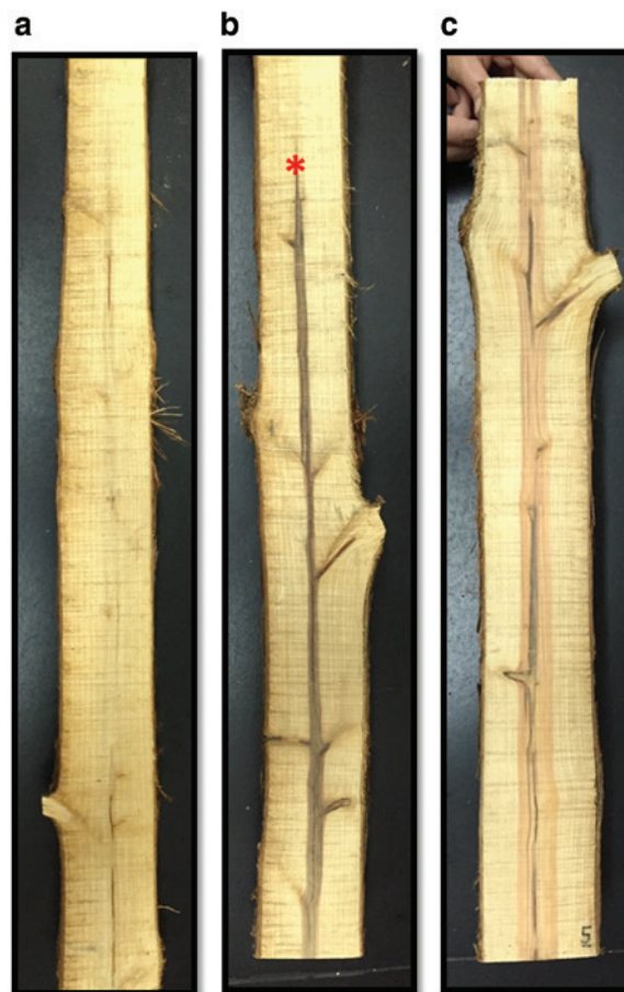
Figure 5: The presence of heartwood formation in Taiwania . (a) log 3 (b) log 4 (c) log 5. The red asterisk indicate the presence of heartwood.
